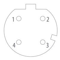
Recommended mating connector type according to IEC 61076-2-10: MM 005-Gx1-B
